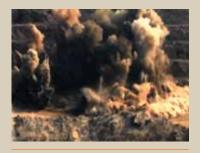
Successful firing with combined production and trim blast at Rampura open cast
