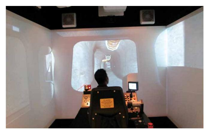
The simulator at Sindesar Khurd mine has a realistic replica of the cabin of actual equipment mounted on a three degree of freedom motion platform, surrounded by 360 degree projection display system and surround sound.
